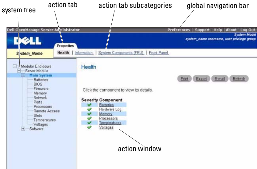
Figure 3-2. Sample Server Administrator Home Page — Modular System
